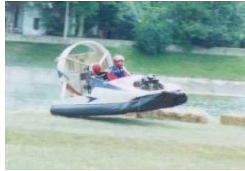
Separate lift and thrust systems
